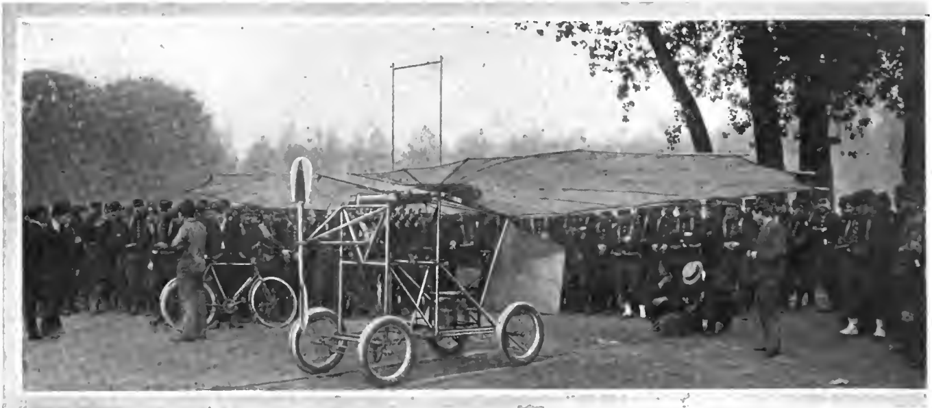
REMODELED AEROPLANE OF M. VUIA, PARIS, NOW FITTED WITH EIGHT-CYLINDER ANTOINETTE MOTOR DRIVING PROPELLER FORWARD.
